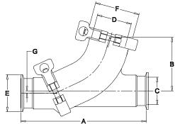
When liquid flows through the valve, the ball is forced into the branch of the valve allowing full fluid flow. When the liquid stops, equalizing the pressure, the ball drops back into the seat, preventing backflow. Should reverse flow occur, the differential pressure will cause the ball to seal firmly against the seat preventing leakage.
